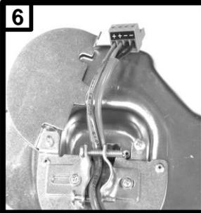
**6** Using a Phillips screwdriver, open the screw on the wiring cover on the rear of the speaker, slide open the cover, and remove the plug-in Phoenix-type connector. Two (2) parallel “-” terminals and two (2) parallel “+” terminals are available for input wiring to the speaker and for output wiring to the next speaker in the string. The wiring schematic for a typical 25V, 70V, or 100V speaker system is shown in the diagram below:
